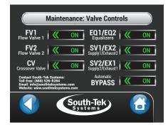
Figure 28: Valve Control Screen
