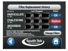
Figure 30: Filter Maintenance Screens
