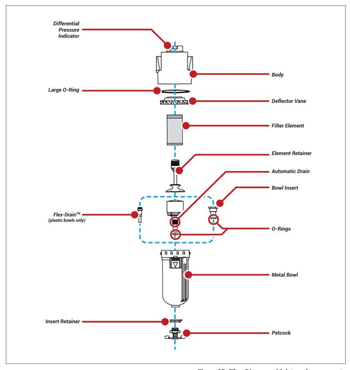
Figure 35: Filter Diagram with internal components
