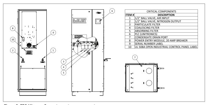
Figure 3: FPS Nitrogen Generator system components
