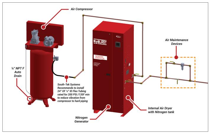
Figure 2: FPS Nitrogen Generator Installation set-up
