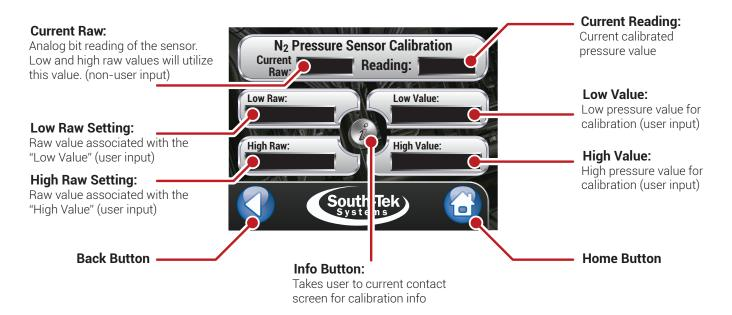
Figure 25: N2 Tank Pressure Calibration Screen Breakout
