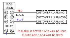
Figure 7: FPS-500 Alarm Contact Diagram
