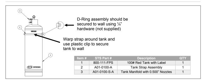
Figure 4: FPS nitrogen tank details and connections
