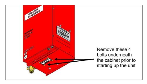
Figure 1: Remove shipping bolts (x4)
