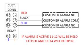
Figure 7: FPS-900 Alarm Contact Diagram
