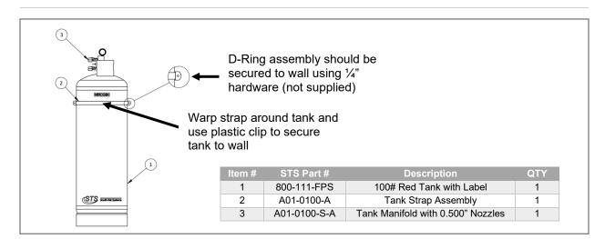
Figure 4: FPS nitrogen tank details and connections
