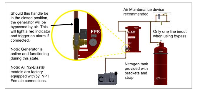
Figure 3: Nitrogen Generator Wall Mount Installation Setup
