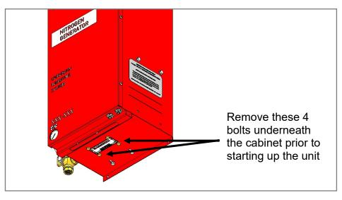
Figure 1: Remove shipping bolts (x4)
