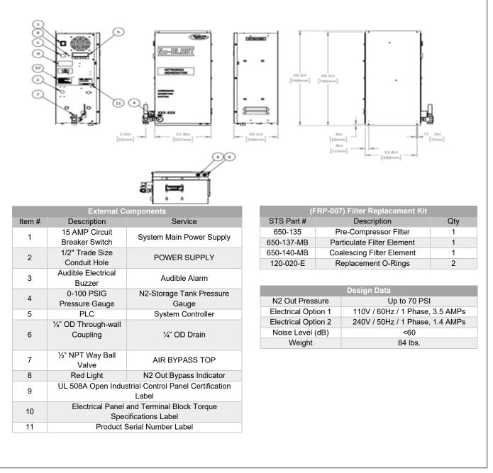
Figure 5: FPS-900 external components and connections
