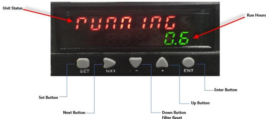
**Figure 1: Controller Display**
