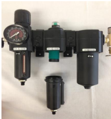
Figure 4: Coalescing Filter Element Replacement
