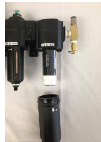
Figure 5: Absorber Filter Replacement
