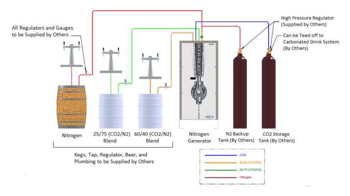
Ports on the upper cabinet are as follows (from left to right): Port 1:  $60/40 CO_2/N_2$  Blend, Port 2:  $CO_2$  In, Port 3:  $25/75 CO_2/N_2$  Blend, Port 4,  $N_2$  Out.
