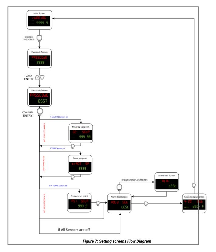
If any of these sensor start alarming an alarm screen will start switches at intervals of 1 second to the current display and it will trigger the buzzer and common alarm contact.
