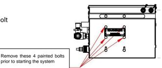
**4.3** UNPACKING AND PREPARATION (BEERBLAST<sup>™</sup> 14KPH AND N<sub>2</sub>-GEN<sup>™</sup> 14KPH)
