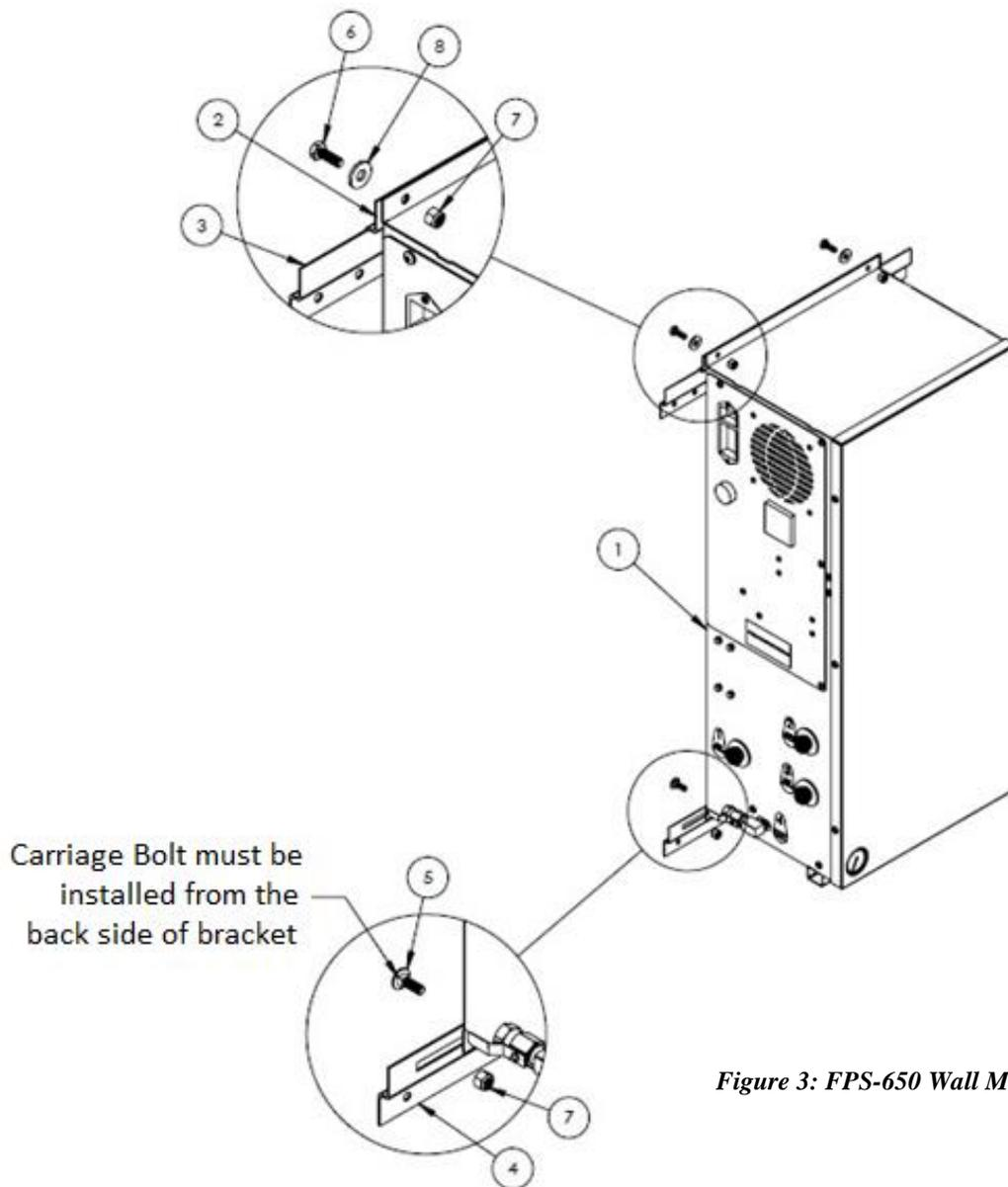
Figure 3: FPS-650 Wall Mounting Diagram
