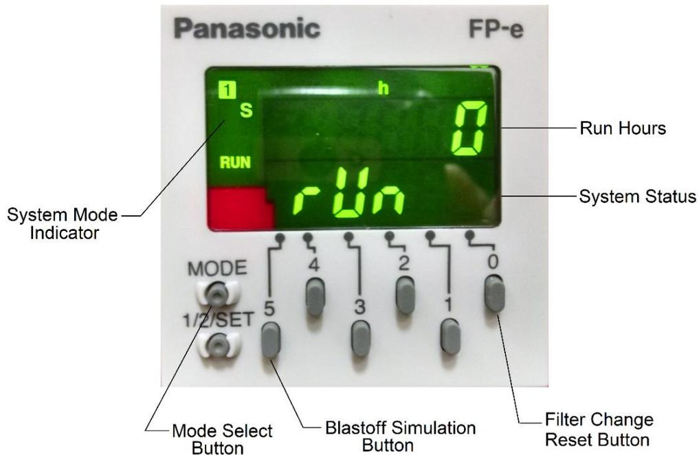
**Figure 1: Controller Display**
