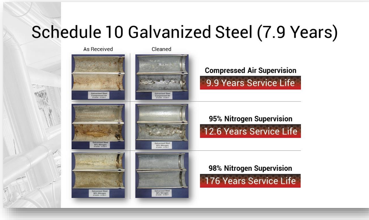
Figure 3. Schedule 10 galvanized steel corrosion test results at 7.9 years.
