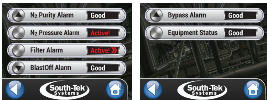
Figure 20: Alarm Menu Screens (O 2 Purity with presence of O 2 Sensor)
