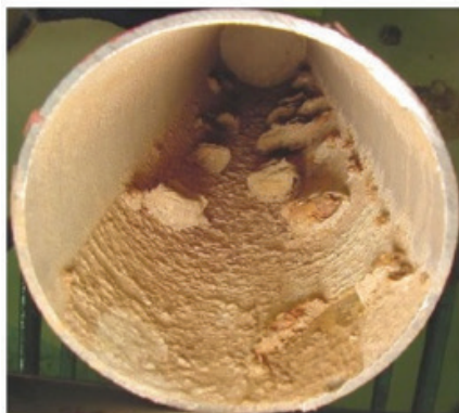
Photograph showing tubercles and pinhole (circled) leakage of galvanized steel sprinkler pipe in dry pipe systems. On left: tubercles heavily formed inside a galvanized steel pipe (4-inch [10-cm] diameter). On right: through-wall (circled) leakage underneath a tubercle (removed) on a galvanized steel pipe. From Research Technical Report, Corrosion and Corrosion Mitigation in Fire Protection Systems , page 28.
