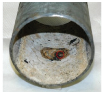
Photograph showing tubercles and pinhole (circled) leakage of galvanized steel sprinkler pipe in dry pipe systems. On left: tubercles heavily formed inside a galvanized steel pipe (4-inch [10-cm] diameter). On right: through-wall (circled) leakage underneath a tubercle (removed) on a galvanized steel pipe. From Research Technical Report, Corrosion and Corrosion Mitigation in Fire Protection Systems , page 28.
