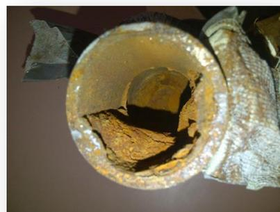
Examples of internal corrosion and corrosion products found in sprinkler pipes for dry and preaction fire protection systems. Photos courtesy of South-Tek Systems.
