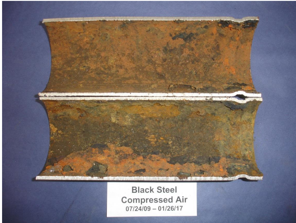
Figure 1. As found condition of interior surface of black steel piping after 2893 days of exposure while half-filled with water and under compressed air supervision.
