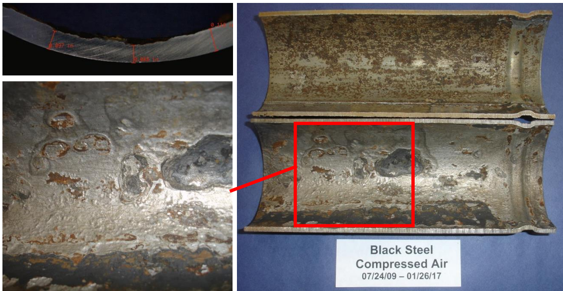
Figure 2. Composite image of cleaned black steel piping after 2893 days of exposure while half-filled with water and under compressed air supervision. Note uniform thinning of pipe wall with a few localized, shallow pits.
