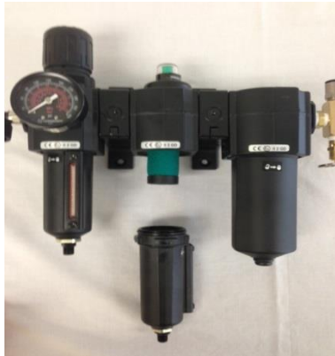
Figure 4: Coalescing Filter Element Replacement
