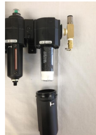
Figure 5: Absorber Filter Replacement
