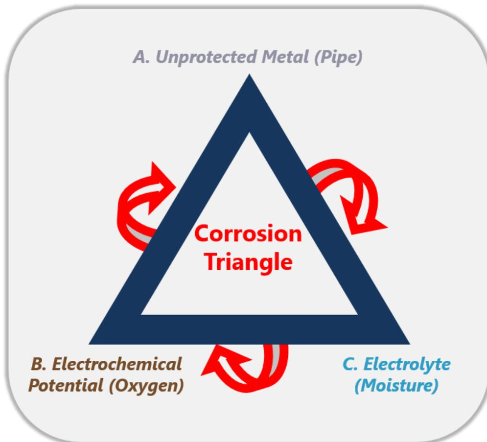
You cannot avoid the metal in this equation. Even in dry and pre-action systems, you cannot dodge the moisture aspect either. Therefore, the most effective way to inhibit the corrosion process is to replace the compressed air (Oxygen) with high purity Nitrogen.
