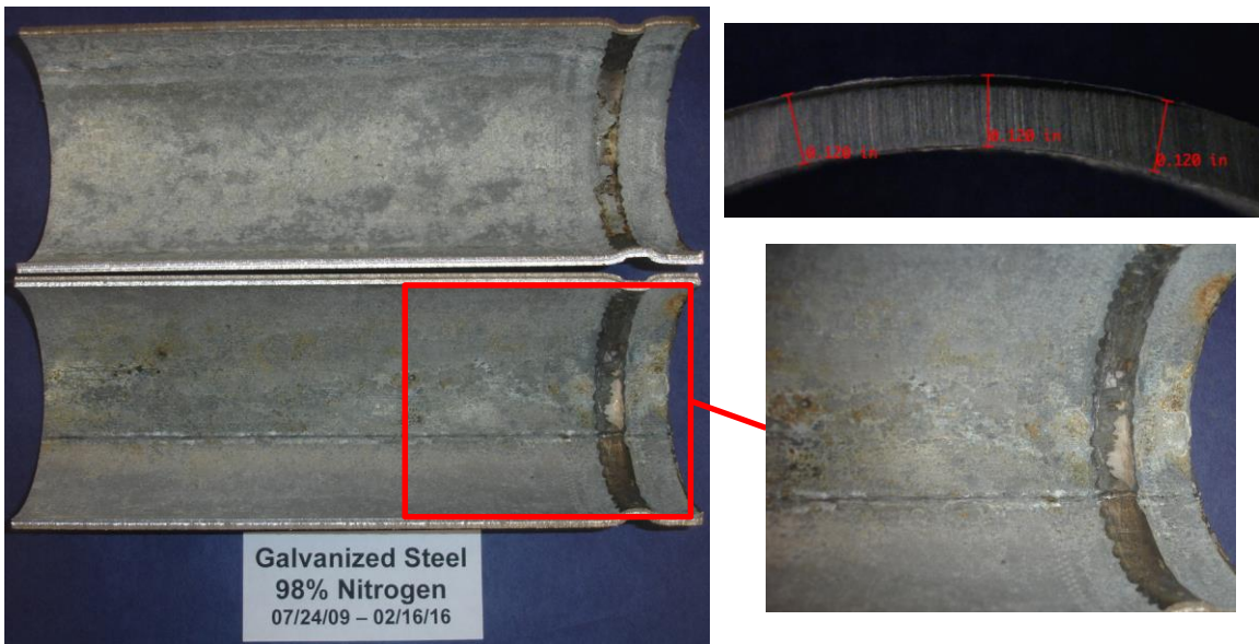
Figure 6. Composite image of cleaned galvanized steel piping after 2398 days exposure while half-filled with water and under 98% nitrogen supervision. Note uniform appearance of pipe wall and absence of any localized pits.
